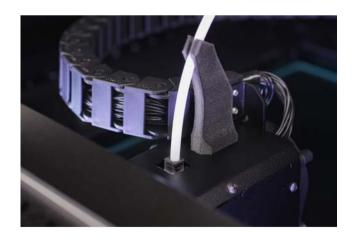
The printhead moves to the parking position: the far left corner. The filament loading is completed.
